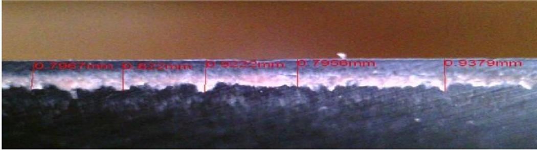
**Figure 10.** A picture of the flank wear width on the blunted blade after performing the experiment
