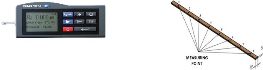
**Figure 4.** TIME3200 roughness meter TIME3200 Surface Roughness Tester TR200 and surface roughness test sample
