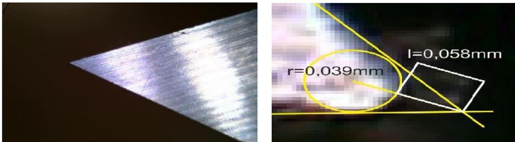
**Figure 11.** Radius of the blade cutting edge
