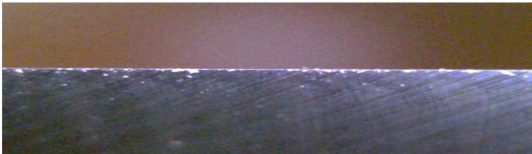
**Figure 7.** A picture of a flank wear width on a newly sharpened blade
