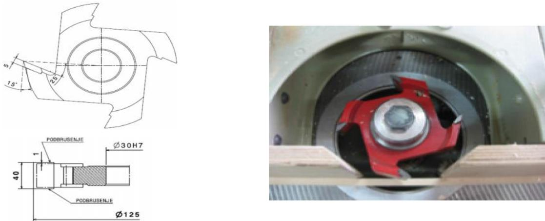
**Figure 2.** A drawing and photo of the tool
