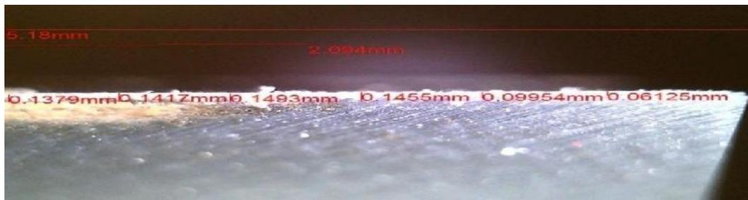
**Figure 9.** A picture of the flank wear width on the blunted blade before starting the experiment
