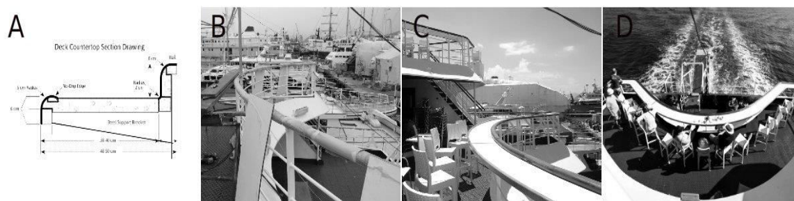
Figure 10a, b, c, d. Upper Deck Back Side Seating Area. Design Proposal – Section Drawing and Realization. Source: Siniša Prvanov
