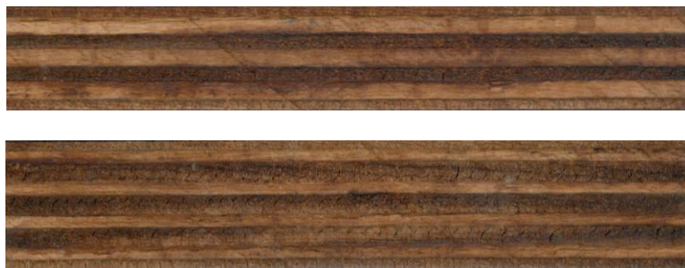
Figure 5. Test specimens of seven and nine-layer plywood models after 6 hours immersion in boiling water
