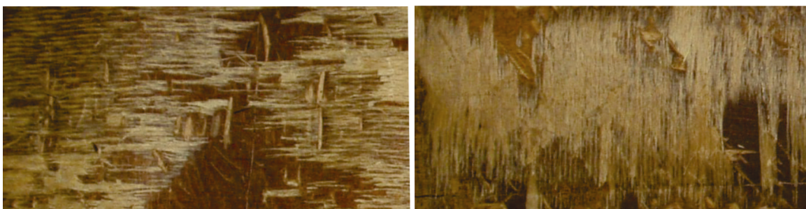
Figure 6. Characteristic wood failure surfaces during determination of the degree of adhesion of plywood models
