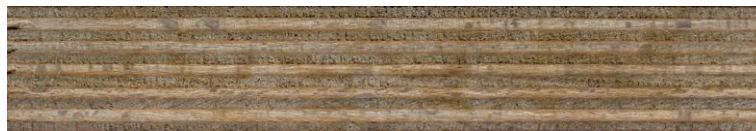
Figure 5. Cross-section of eleven-layer plywood overlaid with phenol-formaldehyde resin impregnated paper after 1248 hours water treatment (model A)
