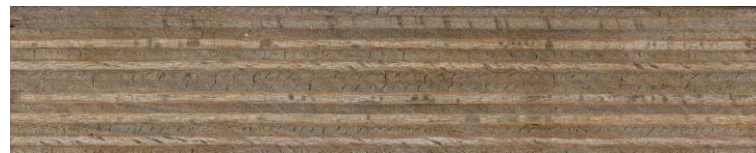
Figure 6. Cross-section of fourteen-layer plywood overlaid with phenol-formaldehyde resin impregnated paper after 1248 hours water treatment (model B)
