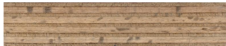
Figure 7. Cross-section of nine-layer plywood without surface protection after 1248 hours water treatment (model C)
