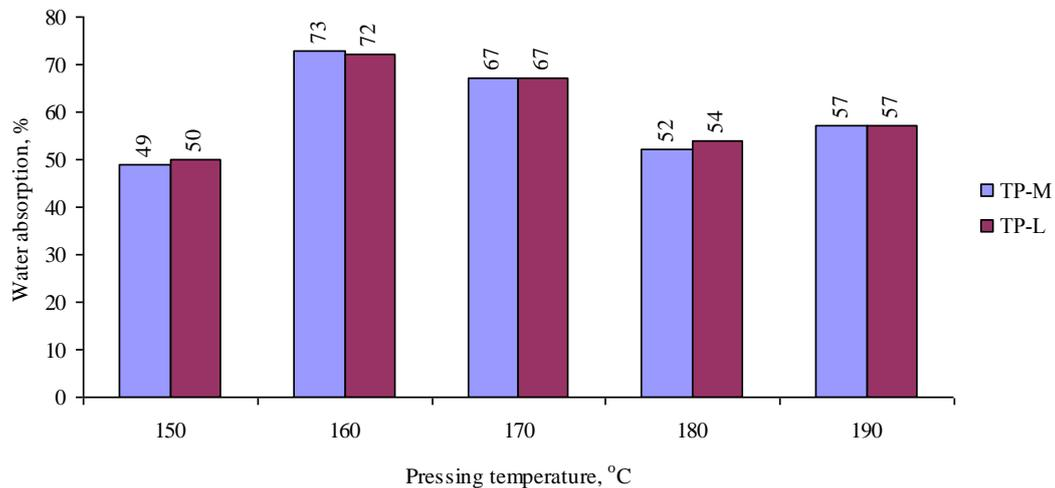
**Figure 1.** Water absorption of panels type TP-M and TP-L at different pressing temperatures
