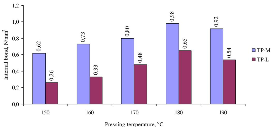
**Figure 4.** Internal bond of panels type TP-M and TP-L at different pressing temperatures
