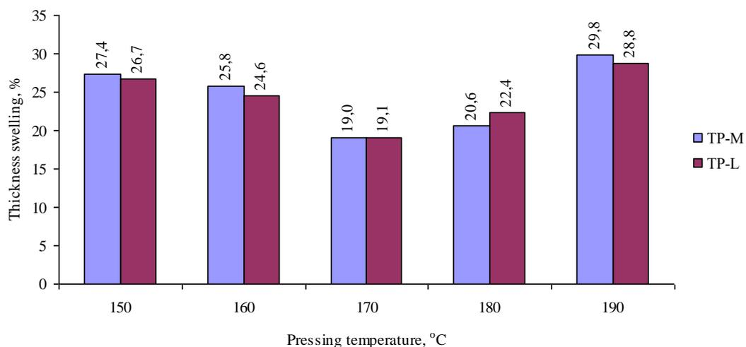
**Figure 2.** Thickness swelling of panels type TP-M and TP-L at different pressing temperatures
