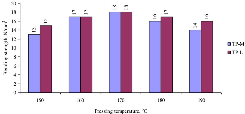
**Figure 3.** Bending strength of panels type TP-M and TP-L at different pressing temperatures
