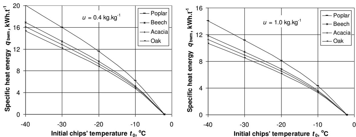
Figure 4. Change in  $q_{bwm}^{m/t}$  of chips with  $u = 0.4 \text{ kg} \cdot \text{kg}^{-1}$  (left) and  $u = 1.0 \text{ kg} \cdot \text{kg}^{-1}$  (right), depending on  $t_0$  and the wood species
