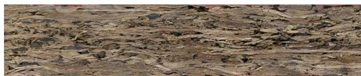
**Figure 7.** Cross-section of oriented strand board (OSB) after water treatment of 1248 hours (control model III)
