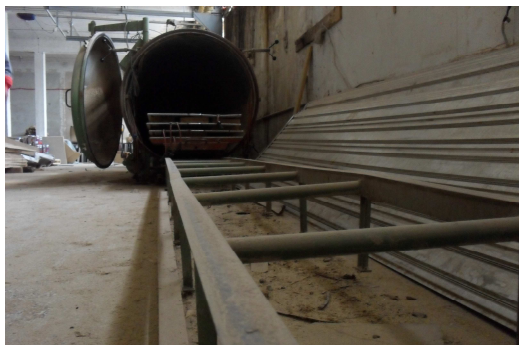
Fig. 4: Vacuum dry kiln
