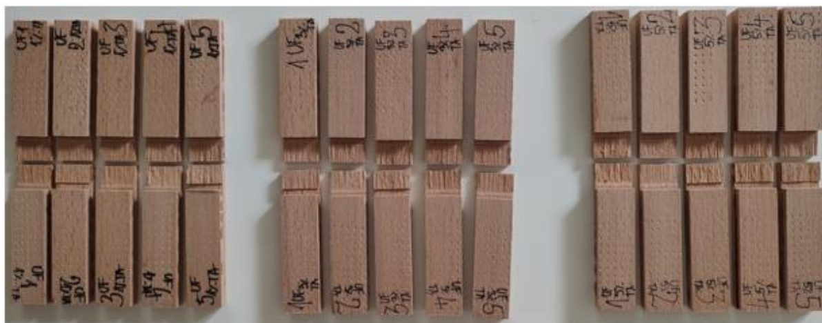
Figure 4. The joint samples underwent complete (100%) wood fracture following tensile shear testing.
