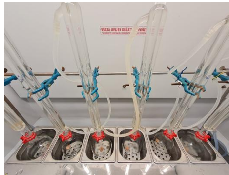
Figure 7. Solid wood samples during extraction.
