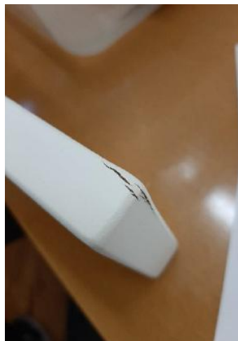
Figure 4. Cracks on narrow edges of coated MDF samples double-faced with ground foil.
