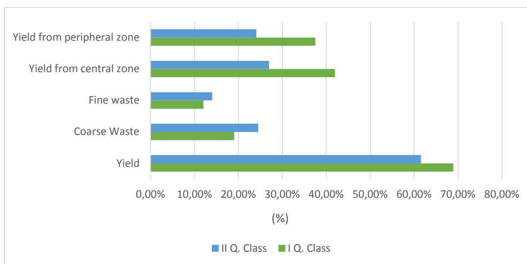
Figure 5. Comparison of yield ( Y_{lumber} , Y_{central} , Y_{peripheral} ), coarse and fine waste in both first- and second-class
