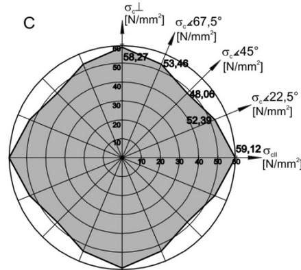
**Figure 3:** Polar diagram of the compressive strength of the control model of plywood without reinforcements
