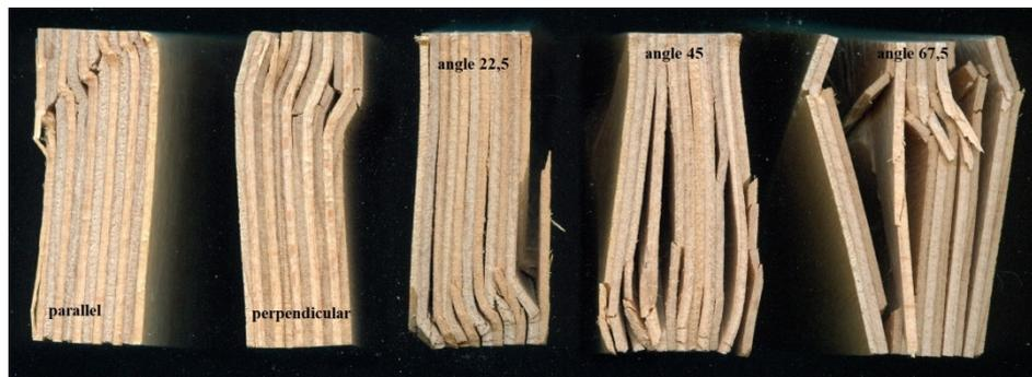
Figure 7: Failure mode of the test specimens of the control model during testing the compressive strength
