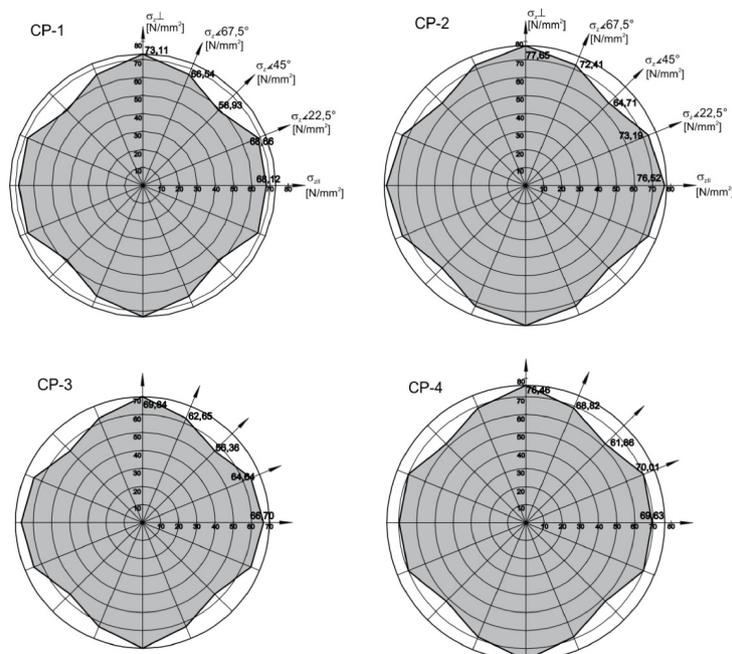
**Figure 2:** Polar diagrams of the compressive strength of plywood reinforced with cotton prepreps
