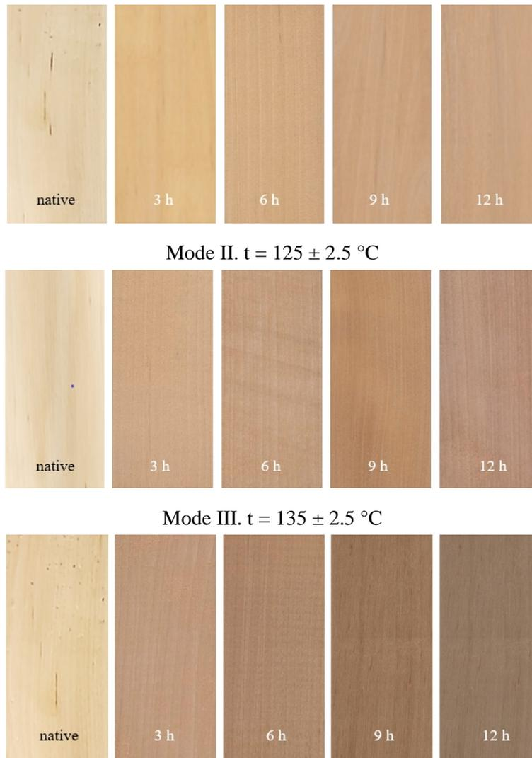
**Figure 2:** Changes in the color of birch wood during thermal modification
