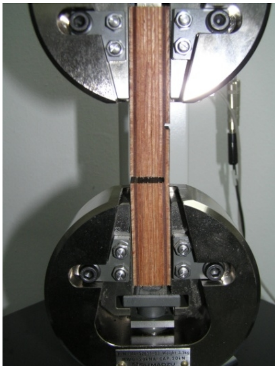
Figure 6. Shear strength test of experimental plywood
