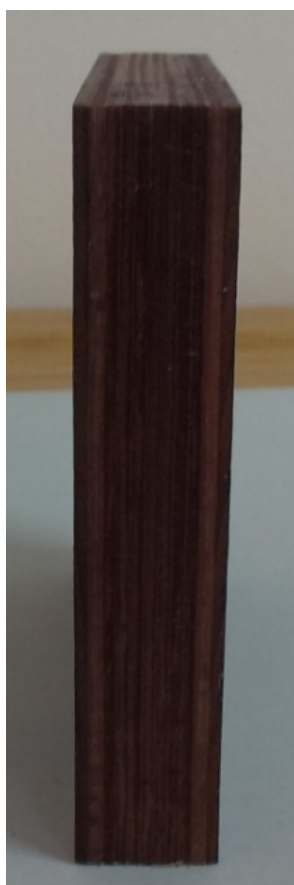
Figure 5. Test specimen of plywood after immersion in water for period of 12 days
