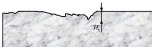
Figure 4. Maximum breakage deposits ( H_i ) of the cutting edge
