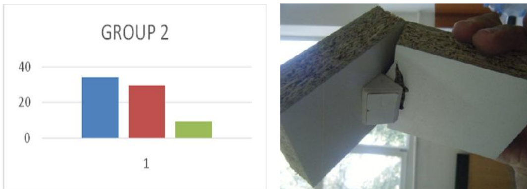
Figure 7. Group 2, specimens taken from the previously tested product (dismounted and then cut off from the product)
