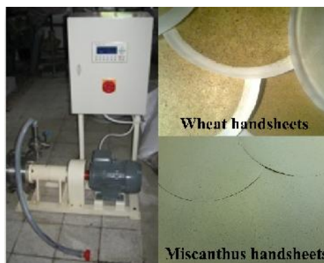
Figure 4. Hydrodynamic cavitation device and agro-waste paper handsheets
