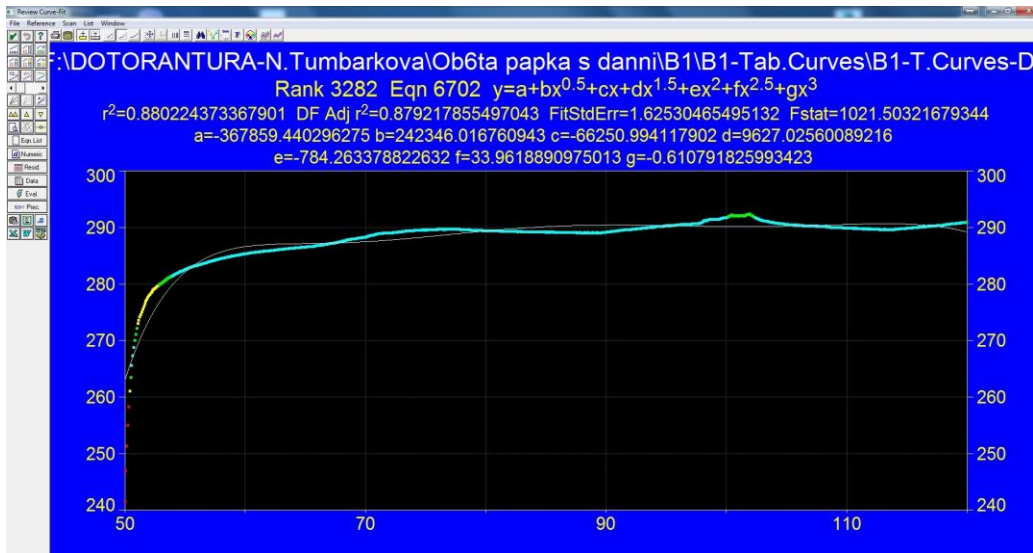
Figure 3. Experimentally established (thick line) and calculated with an equation of 3 rd degree (thin line) change in T_{m-dfr} = f(\tau) when \tau on the abscissa is expressed in hours
