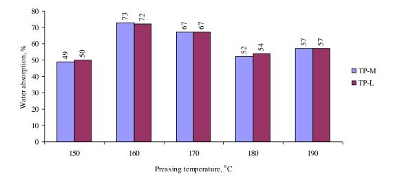
Figure 1. Water absorption of panels type TP-M and TP-L at different pressing temperatures
