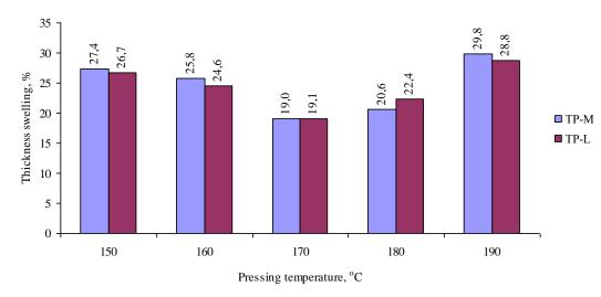
Figure 2. Thickness swelling of panels type TP-M and TP-L at different pressing temperatures
