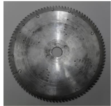
Figure 1. Circular saw with compensating and low noise slots
