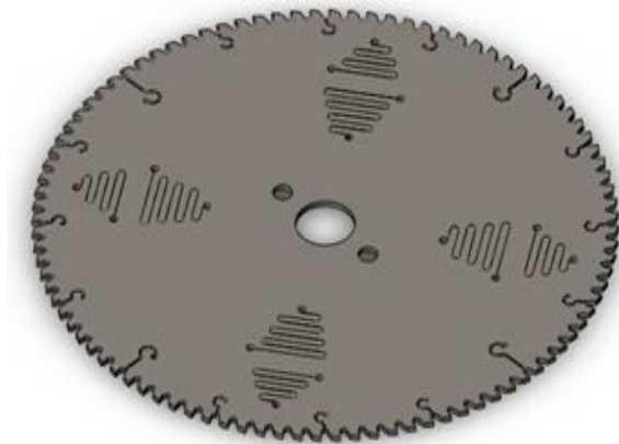
Figure 2. A circular saw with compensating and low noise slots, drawn in 3D
