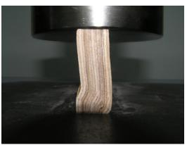
Figure 1: Test specimen during testing the compressive strength of experimental plywood
