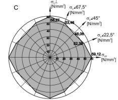
Figure 3: Polar diagram of the compressive strength of the control model of plywood without reinforcements
