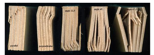
*Figure 7:* Failure mode of the test specimens of the control model during testing the compressive strength
