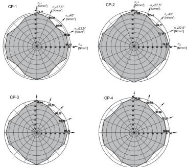
**Figure 2:** Polar diagrams of the compressive strength of plywood reinforced with cotton prepregs In all reinforced plywood models, the highest value of compressive strength is achieved in a direction perpendicular to the face grain, while the lowest value is achieved at an angle of 45° to the face grain of plywood. The biggest difference between the values of compressive strength parallel and
