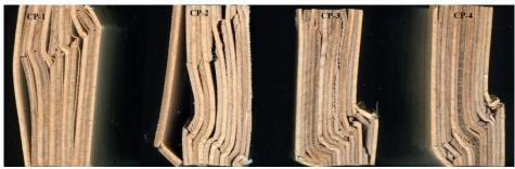
*Figure 6:* Failure mode of the test specimens of reinforced models during testing the compressive strength parallel to the face grain
