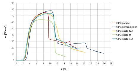
Figure 4: Stress-strain diagram during testing the compressive strength of model CP-2
