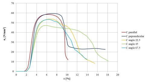
Figure 5: Stress-strain diagram during testing the compressive strength of the control model C
