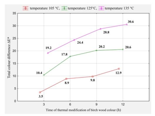
*Figure 3:* Dependence of the total color difference ( *E*\*) on the time of thermal treatment of birch wood
