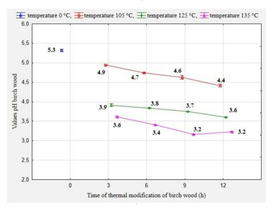
Figure 4: Dependence of birch wood acidity on thermal treatment time
