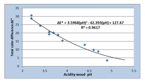
*Figure 5:* The dependence of the total color difference of birch wood ( $E^*$ ) on the acidity value (pH) of wet birch wood in the thermal treatment process
