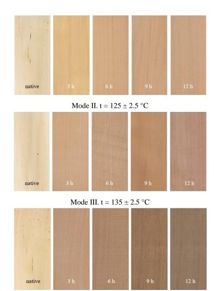
Figure 2: Changes in the color of birch wood during thermal modification
