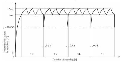
Figure 1. Mode of color modification of birch wood with saturated water steam.
