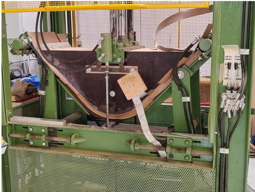
**Figure 5:** Heating specimens and capacitors can be seen added to the press
