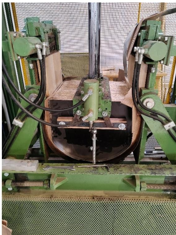
**Figure 2:** Mechanical press during bending
